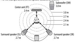
• You can adjust the speaker distance from 0.3 m to 9.0 m. Each time you press the button, the distance changes by 0.3 m.
